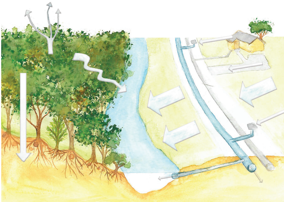
The water cycle. In natural landscapes, water slowly infiltrates into the earth, and runs off into rivers and streams (left). In urban landscapes, it quickly runs off impermeable surfaces (right).
